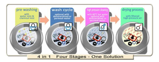
This washing technique is designed in accordance to the practical demands and provides absolute clean washing results with high throughput at short washing and drying process time - with certainty of results ensured! Depending on water quality/cleanliness requirements, a special treatment with demineralized or permeat water is optional possible with an extra module (subsequent upgrade possible).
