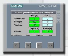
In the user main menu, the operator has all important setting values at one glance. Via comfortable touchpanel, parameters like pre-wash time, high pressure cleaning time, drying time and impulse chemistry can be adjusted. With F1, new set parameter values can be confirmed. With the button F3 you can change to the program mode (recipe administration). Your individual settings can be saved and managed here. By pressing F4, you are directed to the setup mode.
